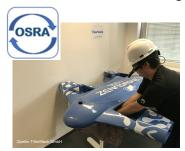
On the data glasses, OSRA-technician is simply started by voice command or touch click. Immediately afterwards, the technician on site is connected to an expert suitable for the respective problem via video call.
